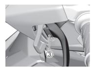
4. Make sure that the brake lever stopper is functioning.
