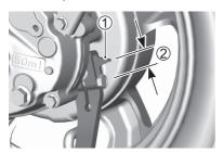
If the indicator is beyond the range, the brake shoe assembly should be replaced by your Suzuki dealer to ensure safe operation.
