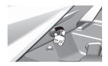
Insert the fuel nozzle ① into the refueling port until it reaches the bottom ②
