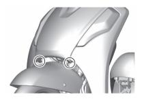
5. Unhook the hooks and remove the front leg shield ①.
