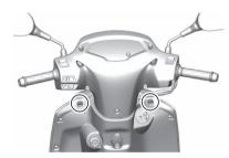
4. Remove the fasteners.
