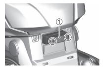
2. Pull off the bulb 2 from the socket.
