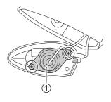
2. Remove the screws and take off the socket ①.
