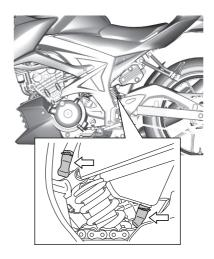
Remove the plugs and drain water and oil at the periodic maintenance interval. The air cleaner drain plugs are located beneath the air cleaner box.
