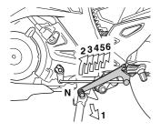
This motorcycle has 6-speed transmission which operates as shown. To shift properly, squeeze the clutch lever and close the throttle at the same time you operate the gearshift lever. Lift the gearshift lever to upshift and depress the lever to downshift. Neutral is located between 1st and 2nd gear. When neutral is desired, depress or lift the lever halfway between 1st and 2nd gear.
