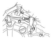
At each maintenance interval, adjust the clutch cable play with the clutch cable adjuster. The cable play should be 10-14 mm (0.4-0.5 in) as measured at the clutch lever end before the clutch begins to disengage. If you find that the amount of clutch cable play is incorrect, adjust it in the following way:
