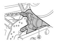
8. Remove the rear brake caliper assembly ④.
