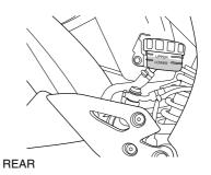
Check the brake fluid level in both the front and rear brake fluid reservoirs. If the level in either reservoir is below the lower mark, inspect for brake pad wear and leaks.
