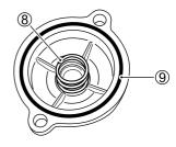
8. Before reinstalling the oil filter cap, be sure to check that the filter spring ® and the "O" ring ® are installed correctly.
