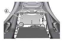
5. Remove the screws and the air cleaner cap 4.
