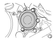
6. Remove the bolts 4 holding the filter cap 5 in place.
