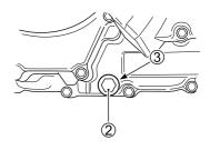
Remove the drain plug 2 and gasket 3 with a wrench and drain out the engine oil while holding the motorcycle vertically.
