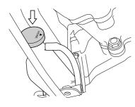
Remove the filler cap and add specified engine coolant through the filler hole until it reaches the "F" line. Refer to the FUEL, ENGINE OIL AND COOLANT RECOMMENDATIONS section.
