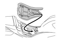
To reinstall the seat, slide the seat hook into the seat hook retainer on the frame and tighten the bolts securely.
