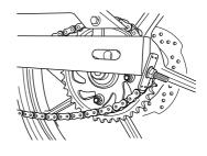
7. With the wheel moved forward, remove the chain from the sprocket.
