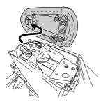
To reinstall the seat, slide the seat hook into the seat hook retainer and push down firmly until the seat snaps into the locked position.
