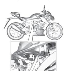
Inspect the fuel hose for damage and fuel leakage. If any defects are found, the fuel hose must be replaced.
