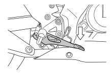
Depressing the rear brake pedal will apply the rear brake. The brake light will be lit when the rear brake is operated.
