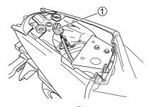
Diagnostic connector 1 is located under the rear seat.
