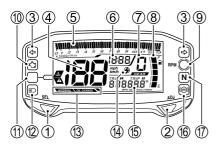
**TURN SIGNAL INDICATOR LIGHT** " $\Longrightarrow$ " ③ When the turn signals are being operated either to the right or to the left, the indicator light will blink intermittently.
