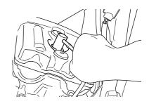
3. Remove the spark plug with a spark plug wrench.
