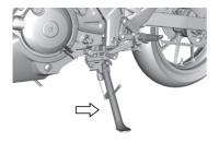
An interlock switch is provided to cut off the ignition circuit when the side stand is down and the transmission is in any gear other than neutral.
