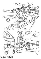
The frame number ① is stamped on the steering head tube. The engine serial number ② is stamped on the crankcase assembly.
