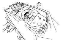
2. Turn the socket ① counterclockwise and remove it.
