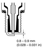
Adjust the spark plug gap to 0.8-0.9 mm (0.028-0.031 in) by using a spark plug gap thickness gauge. The spark plug should be replaced periodically.
