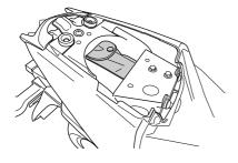
The tool kit is provided with your motorcycle. It is located under the rear seat.
