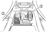
4. Remove the starter relay box ② and the relay box ③.
