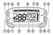
To change the display, push the SEL button ①. The display changes in the order below.
