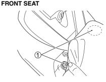
Lift up the rear end of seat and remove the bolts ①.
