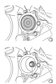
7. Replace the oil filter ⑥ and the "O" ring ⑦ with a new one.
