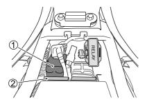
The main fuse is located under the front seat. One 20A spare fuse is located in the starter relay box 1.
