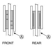
Inspect the front and rear brake pads by noting whether or not the friction pads are worn down to the grooved wear limit line (A). If a front or rear pad is worn to the grooved wear limit line, it must be replaced with a new one by your authorized Suzuki dealer or a qualified service mechanic.
