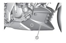
3. Unhook the hook and remove the under cowling ①.
