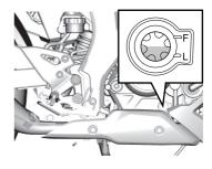
4. Retract the side stand. Hold the motor-cycle vertically and inspect the engine oil level through the engine oil level inspection window on the right side of the engine. The engine oil level should be between the "L" (low) and the "F" (full) lines.
