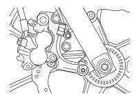
2. Remove the front wheel speed sensor by removing the mounting bolt.
