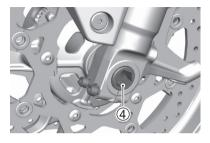
NOTE: A special tool is necessary to loosen the axle shaft ④. The special tool is available at your Suzuki dealer.
