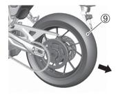
NOTE: Never depress the rear brake pedal with the rear wheel removed. It is very difficult to force the pads back into the caliper assembly.
