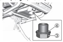
12. Pour 3500 ml (3.7/3.1 US/Imp. qt) of new engine oil through the filler hole and install the filler cap. Be sure to always use the specified engine oil described in the "SELECTING THE ENGINE OIL" section on page 3-25.
