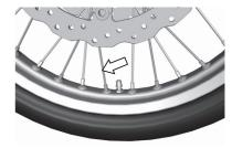
To tighten the spoke nipples properly, tighten them equally to the specified torque. Loosened and overtightened spoke nipples may cause unequal tension of spokes and may result in distortion of the wheel rim. Contact your Suzuki dealer to perform this service.
