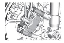
NOTE: Never squeeze the brake lever with the caliper removed. It is very difficult to force the pads back into the caliper assembly and brake fluid leakage may result.
