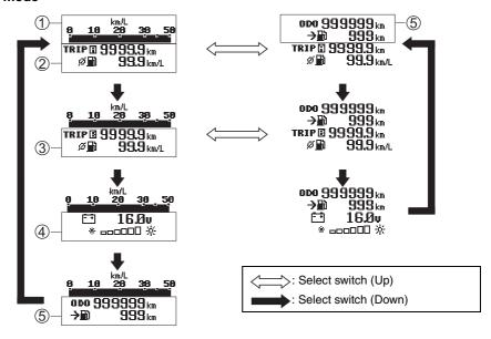
Operate the select switch (Up or Down) to set each item in the multifunction display.
