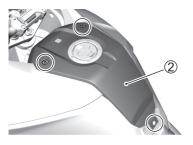
5. Remove the bolts and fasteners. Unhook the hooks and remove the right and left side covers ③.
