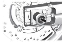
7. With the wheel moved forward, remove the chain **(®)** from the sprocket **(**\bar{T}\).
