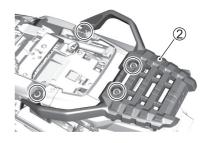
6. Remove the bolts. Remove the right and left side case upper brackets 3.
