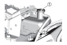
NOTE: Adding only water will dilute the engine coolant and reduce its effectiveness. Add specified engine coolant.
