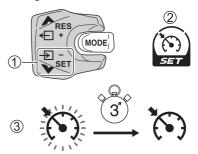
When riding at the target motorcycle speed, press the select switch (RES/+) or select switch (SET/-) to adjust the target motorcycle speed.
