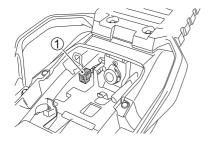
NOTE: The diagnostic connector is used by a Suzuki dealer or a qualified service mechanic.
