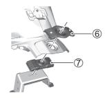
10. Support the fuel tank (8) with the prop (6).
