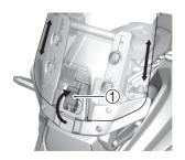
Tilt the windshield lock lever ① downward to lock the windshield.
