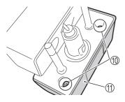
13. Push in on the bulb, twisting it to the left, and pull it out.
