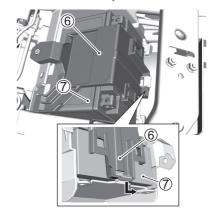
10. Wipe any white powder adhering to the terminal section away with warm water. If there is severe corrosion, buff it off with sandpaper.
