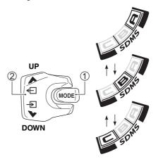
The Suzuki drive mode selector indicator indicates the selected mode. When the MODE switch ① is pressed, the mode selection state is canceled.
