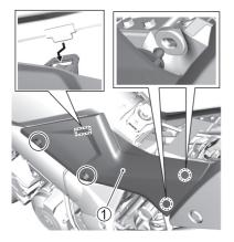
Remove the bolts. Remove the carrier②.
