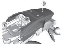
10. Remove the screws. Remove the rear fender and disconnect the lead wire couplers .
