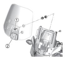
2. Move the windshield nuts ③ up or down to the desired windshield position.
