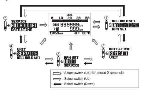
Operate the select switch (Up or Down) to set each item in the multifunction display.
