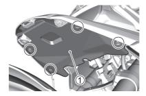
4. Remove the bolts. Remove the fuel tank center cover ②.
