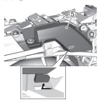
9. Remove the fastener. Remove the frame center cover ⑥.
