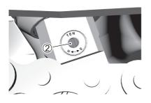
To set the rebound damping force adjuster to the standard position, turn the adjuster clockwise until it stops and then turn it counterclockwise 1-1/4 turn.
