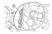
4. Inspect the air cleaner element condition. Replace the air cleaner element periodically.
