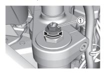
There are 5 grooved lines on the side of the adjuster for reference. Position 5 provides the minimum spring pre-load and position 0 provides the maximum pre-load. This motorcycle is delivered from the factory with its adjuster set on position 4.
