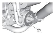
7. Smear a little engine oil around the rubber gasket (8) of the new oil filter.
