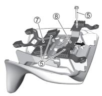
NOTE: Stow the seat frame mounting bolts © removed at step 5 to the adapter mounting bolt © fixing positions on the underside of the rear seat.
