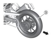
NOTE: Never depress the rear brake pedal with the rear wheel removed. It is very difficult to force the pads back into the caliper assembly.
