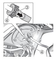
5. Remove the bolt and nut.
