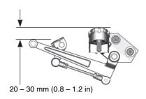
After adjusting, rotate lock nut A and B in the opposite direction of step1 (介) to tighten them.
