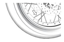
To tighten the spoke nipples properly, tighten them equally to the specified torque. Loosened and overtightened spoke nipples may cause unequal tension of spokes and may result in distortion of the wheel rim. Contact your Suzuki dealer to perform this service.
