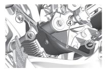
7. Remove the bolts. Unhook the hooks and remove the right and left frame front cover ⑤.
