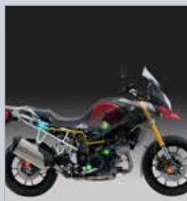
Traction control system
