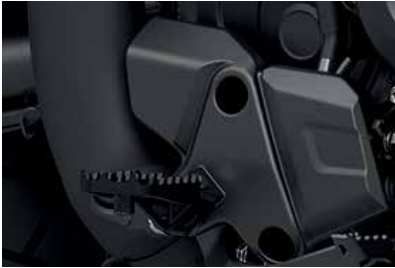
RALLY STEPS 08R72-K3S-JA0 The Rally Step Kit decreases boot slippage by means of a wide tread with an aggressive spike shape. It also further improves stability and control during off-road riding.
