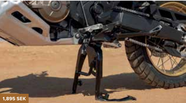
MAIN STAND 08M70-MKS-E00 The Main Stand allows secure parking on a variety of ground surfaces and assists with maintenance operations.
