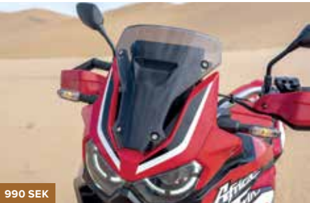
SMOKE WIND SCREEN 8R70-MKS-E00 Add an extra touch of toughness to the front end of your Africa Twin with this smoke wind screen (same shape and dimensions as the standard one).
