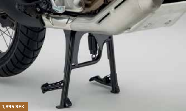
MAIN STAND 08M70-MKS-E00 The Main Stand allows secure parking on a variety of ground surfaces and assists with maintenance operations.
