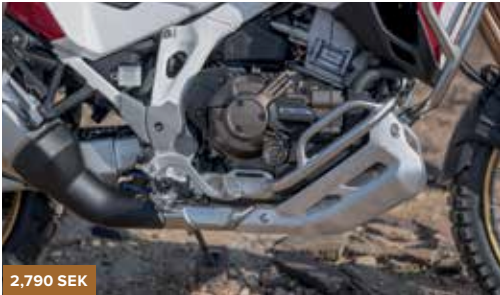
ENGINE GUARD WITH ATTACHMENT 08ESY-MKS-ENG The Engine Guard improve the protection of the engine and the lower part of the bike. Made of stainless steel and finished with electrolytic polishing. This set includes: • Engine guard (08P71-MKS-E00) • Attachment (08P75-MKS-E00)
