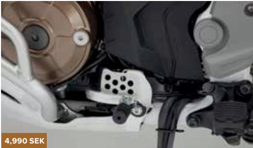
DCT PEDAL SHIFT 08U70-MKS-E50 This kit enables the rider to change gear in the traditional 1 down - 5 up format by using the left foot. It works alongside the handlebar shift triggers giving the rider the choice of using either at any point. (For DCT Version only).
