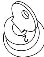
Enables high voltage battery and makes motor ready for operation.
